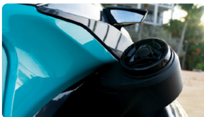
BRP Audio – Premium System (optional) The industry's first manufacturer-installed truly waterproof Bluetooth 2 audio system.
